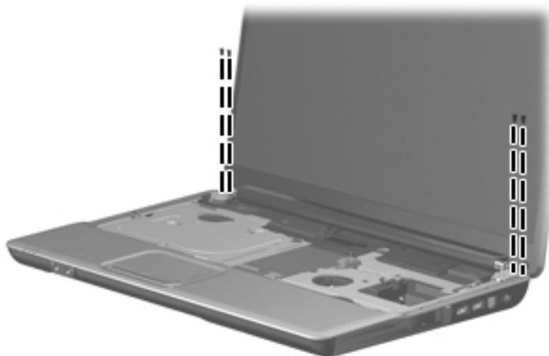
**Where used:** 4 screws that secure the display hinges to the computer
