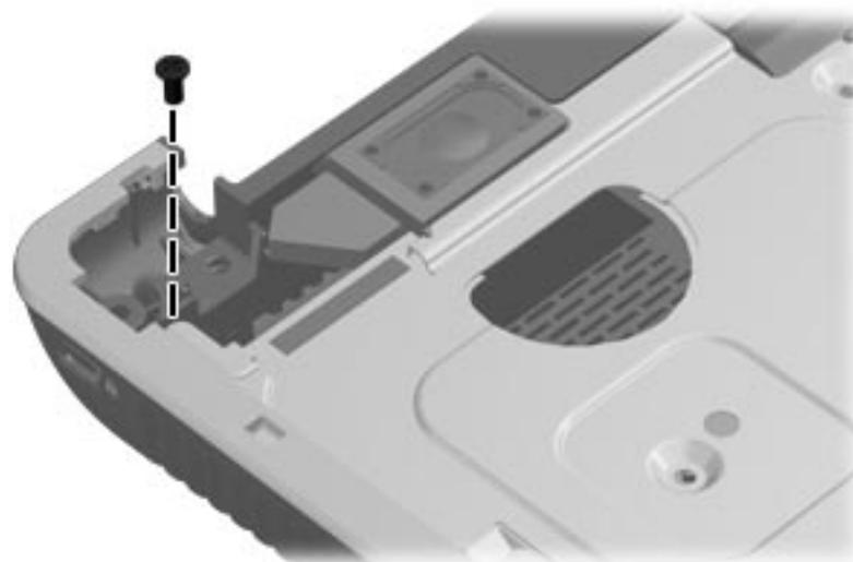
**Where used:** 1 screw that secures the top cover to the computer
