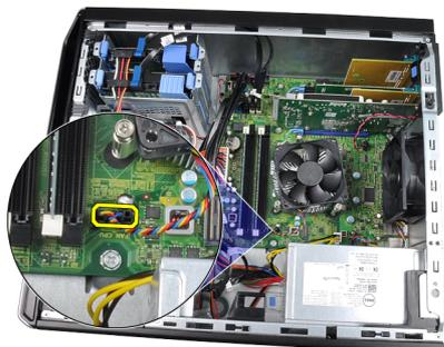
4. Use a Phillips screwdriver to loosen the captive screws securing the heat sink/fan assembly to the system board.
