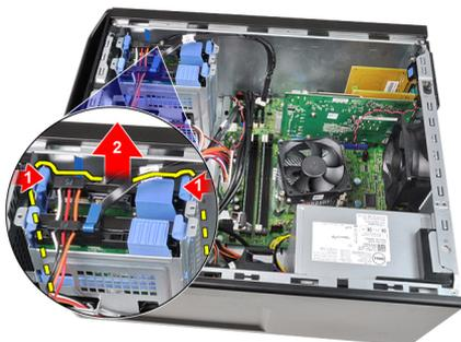
5. Flex the hard drive bracket and then remove the hard drive from the bracket.
