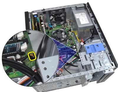
6. Unthread the power switch cable from the chassis clips.
