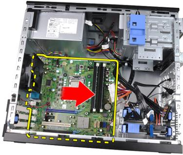
9. Carefully tilt the system board to 45–degrees, and then lift the system board out of the computer.
