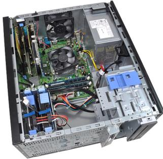
9. Slide the power switch cable out through the front of the computer.
