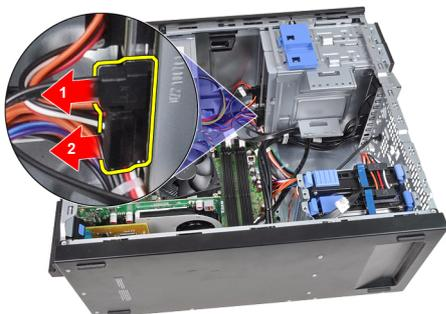
5. Slide down the optical drive latch and then push the optical drive from the back toward the front of the computer.
