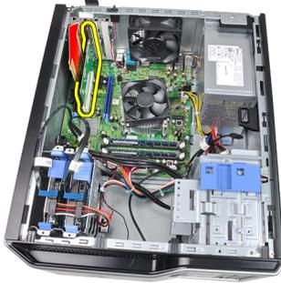
6. Lift the PCI expansion card (if any) up and out of its connector and remove it from the system.
