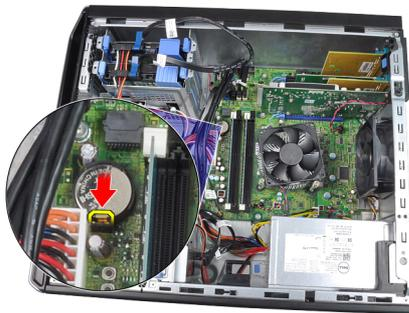
4. Lift the coin-cell battery out of the computer.
