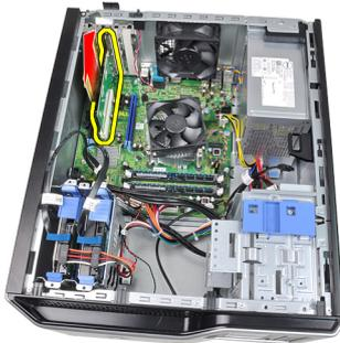
7. Lift the PCI x4 expansion card (if any) up and out of its connector and remove it from the system.
