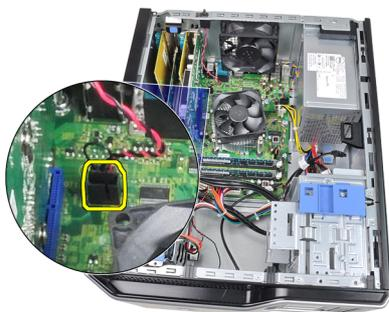
4. Slide the intrusion switch toward the chassis bottom and remove it from the chassis.
