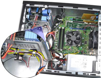
5. Disconnect the 24-pin power cable from the system board.
