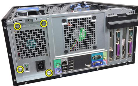
8. Push in on the blue release tab beside the power supply (1), and slide the power supply towards the front of the computer (2).
