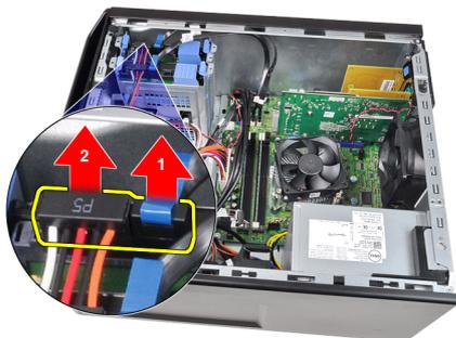
4. Press both blue securing-bracket tabs inward and lift the hard drive bracket out of the bay.
