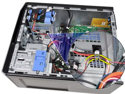
5. Press down the speaker-securing tab and slide the speaker upwards to remove.
