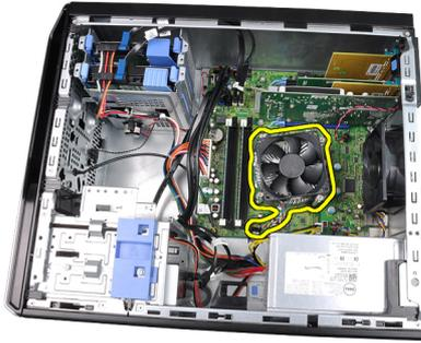
6. Press the release lever down and then move it outward to release it from the retention hook that secures it.
