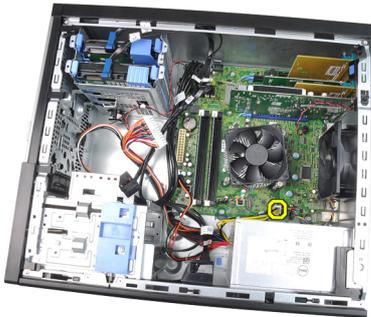
7. Remove the four screws securing the power supply to the back of the computer.
