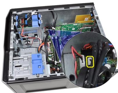
4. Unthread the thermal sensor cable from the chassis clip.
