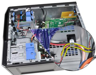
5. Gently pry the thermal sensor away from the chassis front and remove.
