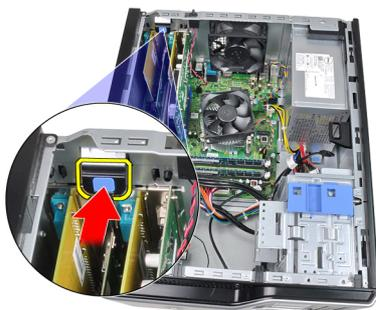
4. Gently pull the release lever away from the PCIe x16 card until you release the securing tab from the dent in the card. Then, ease the card up and out of its connector and remove it from the system.
