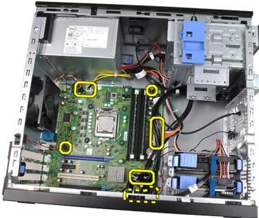
7. Remove the screws that secure the system board to the computer.
