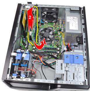
5. Lift the PCIe x1 expansion card (if any) up and out of its connector and remove it from the system.
