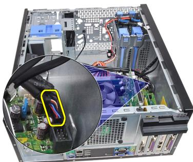
5. Unthread the I/O Panel and FlyWire cable from the clip on the computer.
