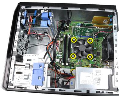
5. Lift the heat sink/fan assembly upward gently, and remove it from the system. Lay the assembly with the fan facing downward, and with the thermal grease facing upward.
