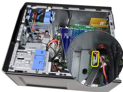
4. Unthread the internal speaker cable from the chassis clip.
