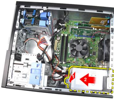
9. Lift the power supply out of the computer.
